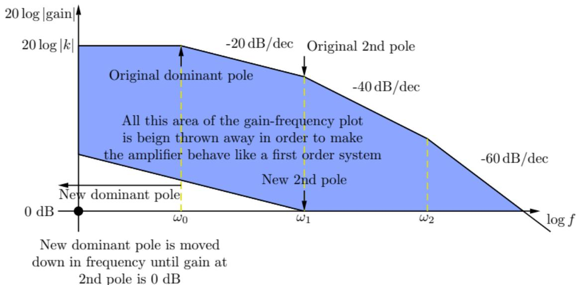
The dominant pole is moved down in frequency (sometimes called “slugging”) until the 2nd pole frequency is at the unity gain point ( $0 \text{ dB}$ ). The blue area is open loop gain which is *lost*.
