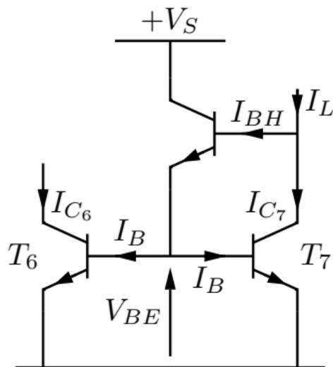
For small signals,  $h_{FE}$  becomes  $\beta$  and the small signal Early resistance of  $T_7$ ,  $r_{ce}$  conducts a small part of  $i_L$  into the negative rail.
