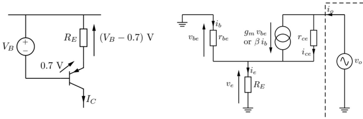
The effective resistance looking into the current source output – its output resistance – will become the new  $R_{VA}$ . For analysis see handout “Small Signal Output Resistance of a Simple Current Source”. In brief  $r_o \approx r_{ce} (1 + \beta)$ .
