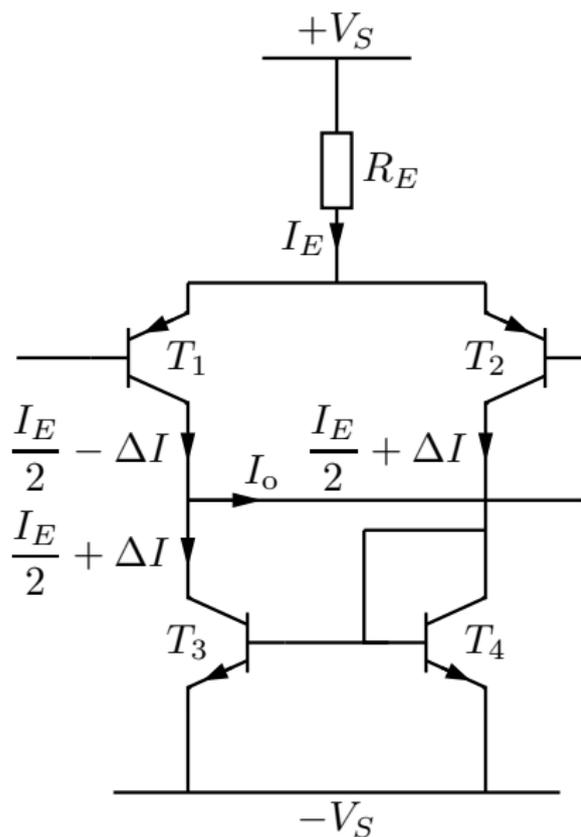
Suppose  $T_1$ 's base is slightly positive with respect to  $T_2$ 's. Considering the action of the current mirror we can sum currents at the collector of  $T_3$ .
