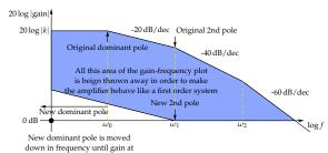
The dominant pole is moved down in frequency (sometimes called "slugging") until the 2nd pole frequency is at the unity gain point (0 dB). The blue area is open loop gain which is lost.
