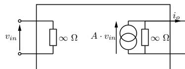
But, the transistor only has three terminals. For the circuits in this course the emitter terminal is common to both the input and output networks. The small signal model of a transistor reduces to,
