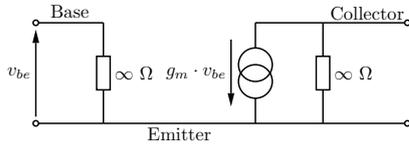
this is a good low frequency model for JFETs, MOSFETs and Valves. The BJT is special however because there is recombination of carriers in the base region, a base current flows. As a result the resistance looking into the base towards the emitter must be finite (by Ohm's law). The characteristics can be used indirectly to yield the small signal base emitter resistance,  $r_{be}$ .
