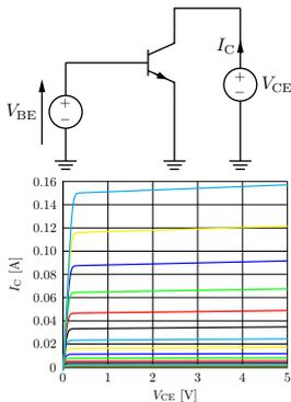
A family of curves showing effect on the output  $V_{CE}$  and  $I_C$  as a function of the input  $V_{BE}$  (or  $I_B$ ). When  $V_{CE}$  is small the transistor is in saturation both BE and CB junctions forward biased (transistor switched "on") (left of graph). When  $V_{BE}$  is too small to cause  $I_C$  to rise above the leakage current level, the transistor is off ( $y \approx 0$  on the graph). Forward active region is indicated by nearly parallel characteristics.
