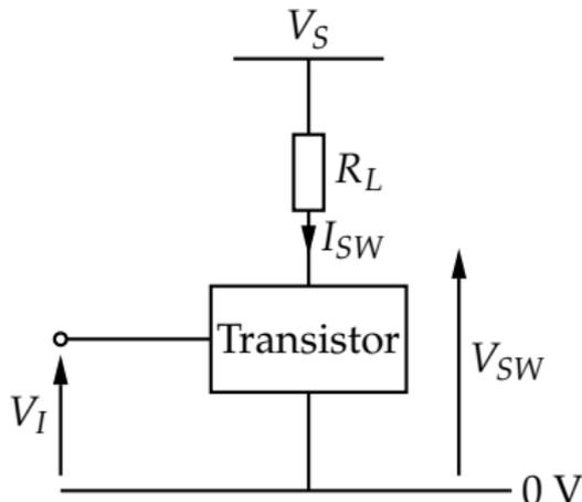
There is also a second relationship between  $V_{SW}$  and  $I_{SW}$  defined by the output characteristics of the transistor.
