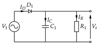
The key elements of **source**,  $V_1$ , **diode**,  $D_1$ , and **capacitor**,  $C_1$ , are connected in series and it is quite common to find a resistor,  $R_1$ , in parallel with the capacitor. The source may be a transformer secondary as is common in radio circuits or an amplifier output as is more typical of instrumentation systems. The circuit has **two distinct states** based on the conduction or non-conduction of the diode.
