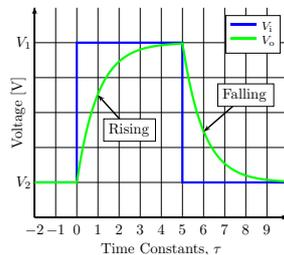
Rising:  $V_o(t) = (V_1 - V_2) (1 - \exp(-\frac{t}{\tau})) + V_2$ ,  $t = 0$  at the start of the pulse
