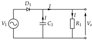
Since the diode is not conducting, replace with open circuit
