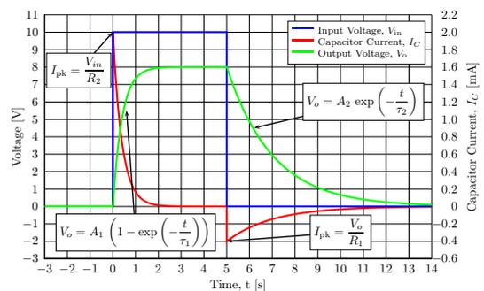
$I_C$  changes direction, hence negative values.  $\tau_2$  is larger than  $\tau_1$ . The negative peak current is given by Ohm's law using the voltage across  $C_1$  at  $t = 5$  s and  $R_1$ .  $I_{pk} = -\frac{7.999}{20 \times 10^3} = -399.95 \mu A$ .
