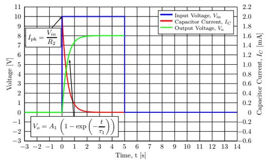
$A_1$  is 8 V in this case and  $I_{pk}$  is 2 mA.  $\tau_1$  the **time constant** is determined by the components involved  $\tau_1 = (R_2 // R_1) C_1$ . The expressions for exponential rise to maximum and exponential decay are derived in the handout.
