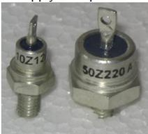
Breakdown voltage from 3 V to 300 V at power ratings of ~mW to 100 W are available. Breakdown voltage tolerance of 5% is common.
