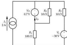
The open circuit must be replaced with a 0.7 V perfect voltage source. Each of the three sources ( $I_1$ ,  $V_1$  and  $V_D$ ) must be considered individually and superposition used to find the current,  $I_D$ , flowing in the forward biased diode.
