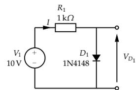
In this simple series diode resistor circuit the diode will limit the current to 9.3 mA. This improved model is often used.
