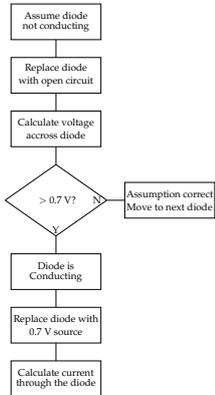
This flow diagram assumes the diode is not conducting. It is equally acceptable to assume that the diode is conducting and construct a slightly different flow diagram. In circuits containing more than one diode, the order in which they are analysed may be important. It is necessary to check that each prior diode every time one is found to change state.
