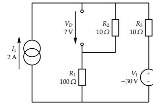
Use the **superposition theorem** to find the **voltage across this open circuit**. If the voltage is **greater than 0.7 V** then the non-conducting assumption is invalid. If the voltage is **less than 0.7 V** the non-conducting assumption is valid and we can state the **reverse bias voltage**. If the **voltage is exactly 0.7 V** the diode will be on the point of conduction and **no current will flow**.
