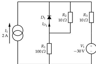
The node voltage and loop current methods and superposition theorem can be used. In this example Ohm's law and superposition will be used.
