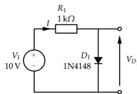
In this diode resistor circuit the resistor limits the current to 10 mA. In this model, the diode is incapable of dissipating power!
