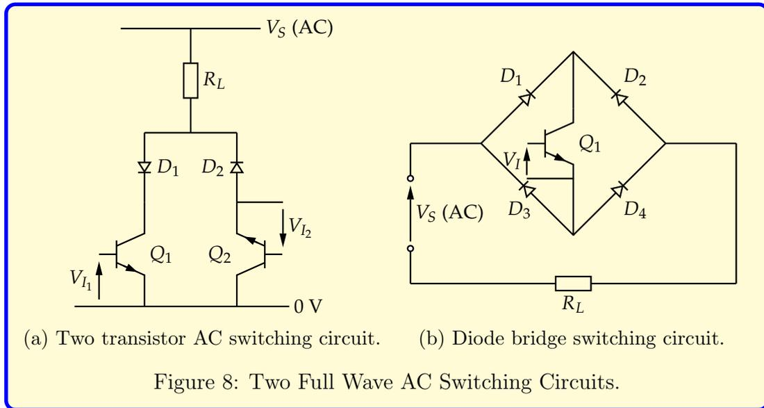
wave approach is to use the four diode bridge with a single switch shown in Fig. 8b. The diode bridge ensures that whatever the instantaneous polarity of  $V_S$ ,  $I_C$  is always in the same direction. The current through  $R_L$  alternates. This circuit has similar difficulties with the control input terminals, but a suitable control circuit is relatively straightforward.
