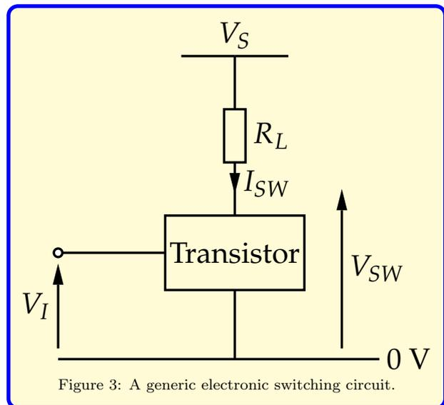
Figure 3: A generic electronic switching circuit.
