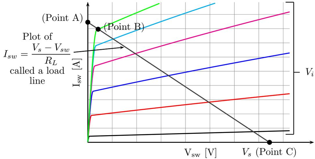
Figure 4: Example of Transistor Output Characteristics.
