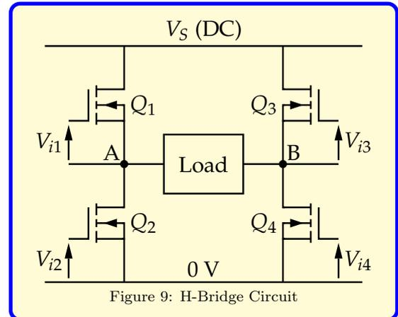
To understand the operation imagine Q1 and Q4 are “on”. Current will flow through Q1 to A, through the load to B and then through Q4. Current can be made to flow from B to A by switching “off” Q1 and Q4 and switching “on” Q3 and Q2. Note if Q1 and Q2 or Q3 and Q4 are ever permitted to be on simultaneously, a large “shoot-through” current will flow and, if there is nothing else to limit the current, the switches will be destroyed, usually very violently.
