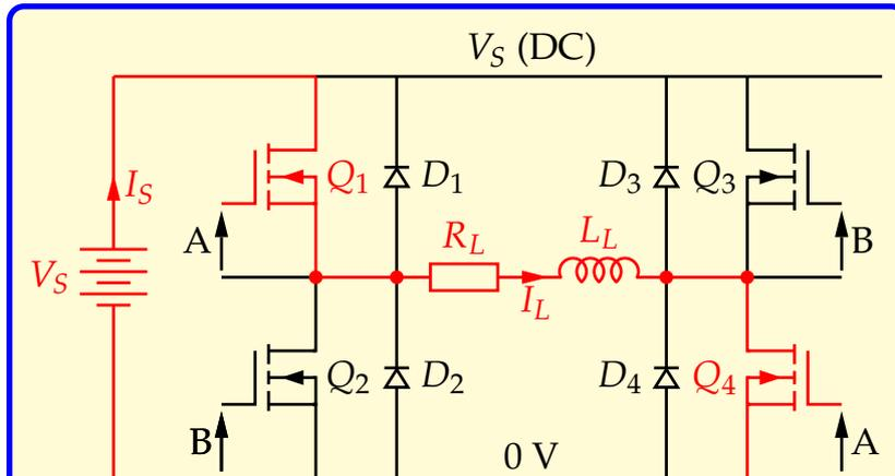
Figure 11: H-bridge with free wheeling diodes, switches conducting.
