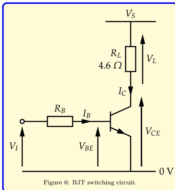
Figure 6: BJT switching circuit.
