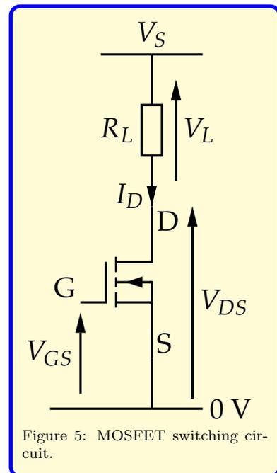
Figure 5: MOSFET switching circuit.
