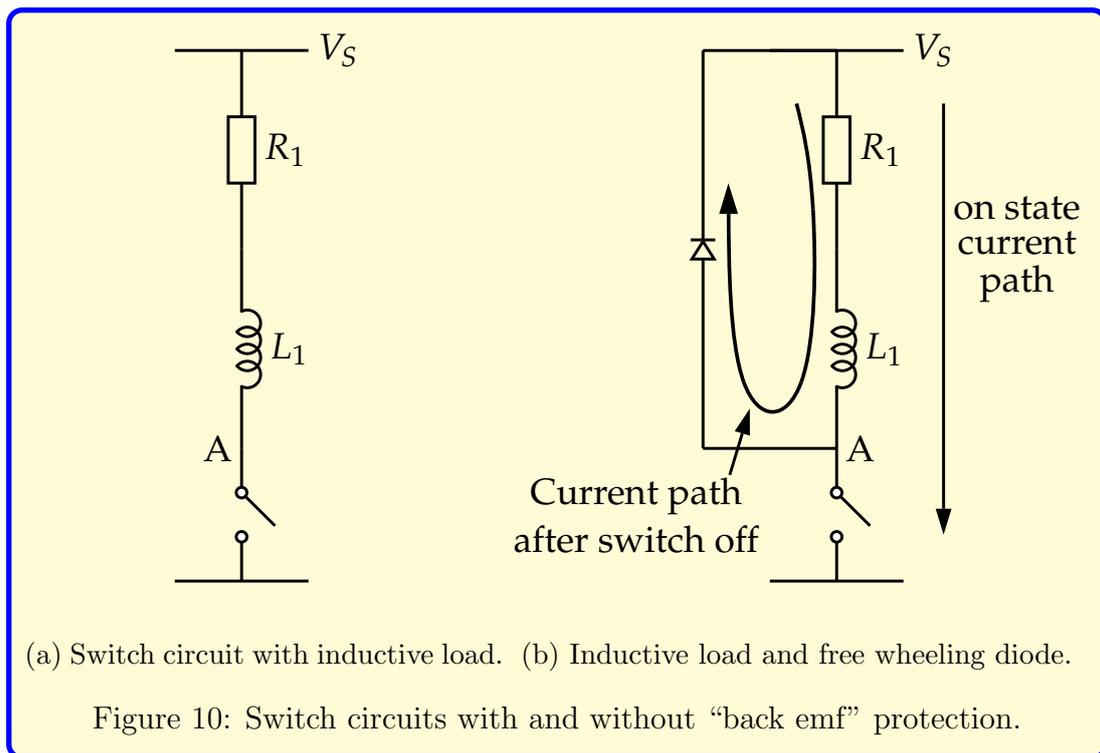
In some applications, these back emf spikes are useful. Examples include car ignition, electric fences, flyback converters (a kind of switched mode power supply), and CRT and VFD display power supplies. In most applications however attempts are made to control them.
