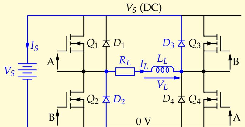
Figure 12: H-bridge with free wheeling diodes, diodes conducting.
