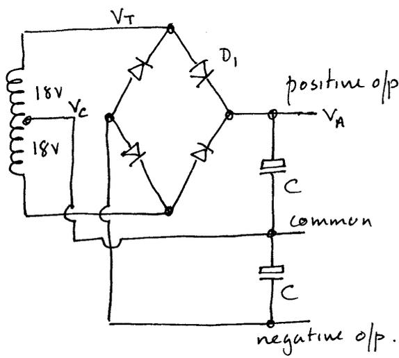
(ii) using the same approximations as in Q2 but recognising that  $I_L$  is given explicitly and the circuit is full wave (ie the charging interval is  $1/2f_s$ )
