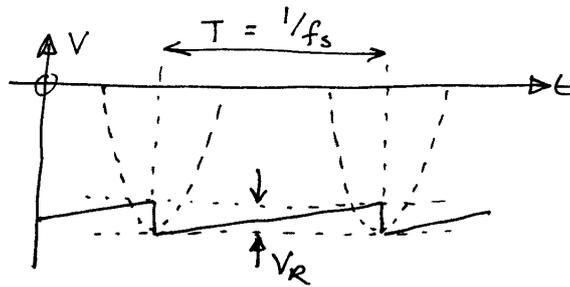
Ripple behaviour governed by  $I_L = C \frac{dV_o}{dt}$  and since  $I_L = \text{const}$ ,  $\frac{dV_o}{dt}$  is the slope of the straight line,  $V_R/T$
