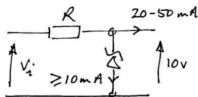
The answer given here uses the instantaneous minimum value of  $V_o$  taking diode drop and ripple into account....
