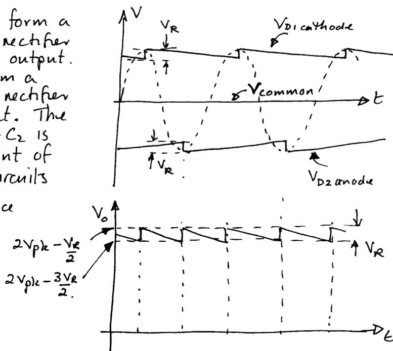
(ii) The  $V_R$  on  $V_o$  is the same in pk-pk value as the  $V_R$  on the output of each half wave rectifier.
