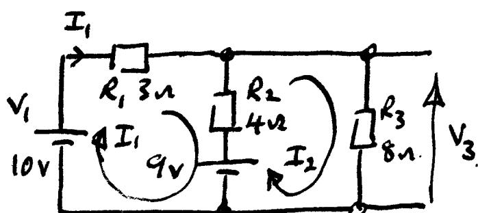
$$10 = I_1 R_1 + (I_1 - I_2) R_2 + 9 \quad \text{--- } ①$$
