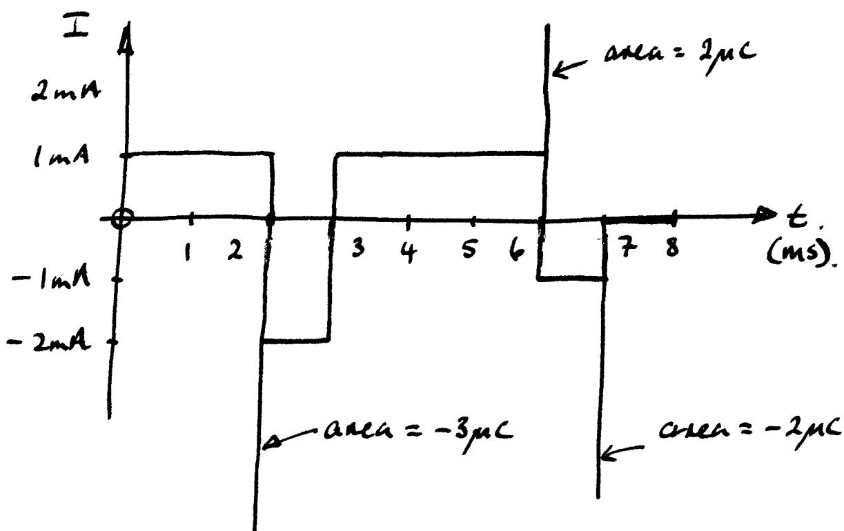
$$0\text{ms} \rightarrow 2\text{ms}, \frac{dV}{dt} = 10^3, I = 1\text{mA}.$$
