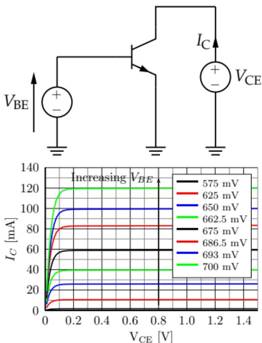
A family of curves showing effect on the output  $V_{CE}$  and  $I_C$  as a function of the input  $V_{BE}$  (or  $I_B$ ). When  $V_{CE}$  is small the transistor is in saturation both BE and CB junctions forward biased (transistor switched “on”) (left of graph). While  $V_{BE}$  is too small to cause  $I_C$  to rise above the leakage current level, the transistor is off ( $y \approx 0$  on the graph). Forward active region is indicated by nearly parallel characteristics.
