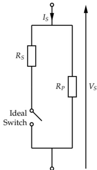
Real switches have some series resistance and some leakage current in the “off state”. In most cases,  $R_P$ , which represents the “off” state leakage can be neglected.  $R_S$  usually has to be considered because it is responsible for the power loss ( $I^2 R$ ) in the switch. For a real switch,
