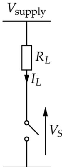
The product of  $V_S$  and  $I_L$  is zero in both switch states so no power is dissipated in the switch.  $I_L$  - the on state current - is determined by the external circuit not the switch.
