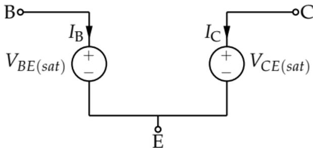
In saturation  $I_C = h_{FE} I_B$  *does not apply*. A model for the transistor when it is off is open circuit between B, C and E. In practice very small leakage currents flow, which are defined on the transistor datasheet.
