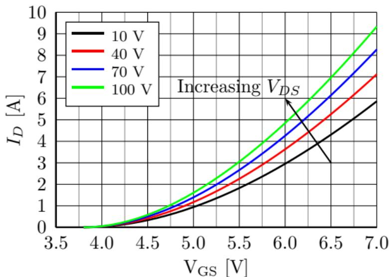
The characteristics of MOSFETs are often found in datasheets, because the transconductance depends on device geometry. In BJTs an expression exists independent of device dimensions.
