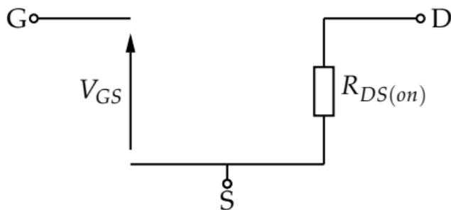
In the linear region the MOSFET behaves like a resistance,  $R_{DS(on)}$ . The value of  $R_{DS(on)}$  is sensitive to temperature (increasing temperature increases  $R_{DS(on)}$ ) however in saturation the dependence is somewhat more complex, based on both the kind of MOSFET (lateral or vertical) and the region of the characteristics it is being operated over.
