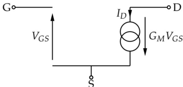
$G_M$  is the large signal transconductance. It is rarely necessary to
