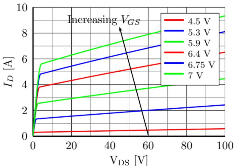
Notice  $V_{GS}$  is much greater than in the BJT case. In the switching region (left) the curves can be assumed parallel,  $R_{DS(on)} \approx$  constant. These characteristics at 25 °C. Very generally speaking  $V_{DS(on)} < V_{CE(sat)}$ .
