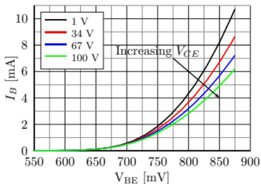
Shape of characteristics essentially governed by the diode equation when  $V_{CE} \approx 0$ .
